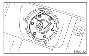
7) Remove sub fuel level sensor.
