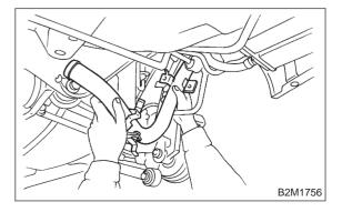
6) Disconnect evaporation hoses from shut valve.
