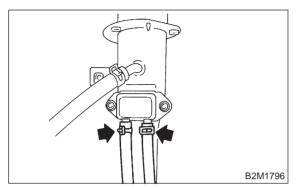
7) Remove shut valve from fuel filler pipe.
