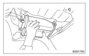
4) Disconnect connector from drain valve.
