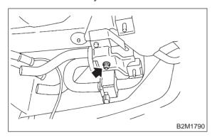
7) Move air filter to upper side, and remove drain valve with bracket.
