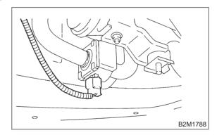
5) Disconnect evaporation hoses from drain valve.
