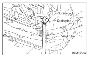
3) Loosen drain cock to drain engine coolant into container.
