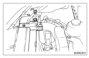
2) Fill engine coolant into radiator up to filler neck position.
