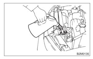
3) Fill engine coolant into reservoir tank up to upper level.
