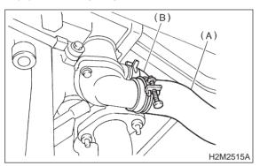
12) Connect connectors to radiator main fan (A) and sub fan (B) motors.
