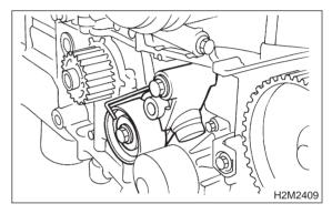
8) Install timing belt. <Ref. to 2-3a [W2C0].> and <Ref. to 2-3b [W2C0].>
