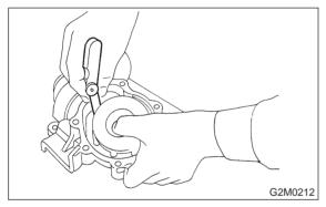
5) After water pump installation, check pulley shaft for engine coolant leaks. If leaks are noted, replace water pump assembly.
