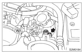
15) Remove left-hand camshaft sprockets by using ST.
