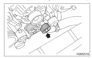
7) Install automatic belt tension adjuster which tension rod is holded with pin.
