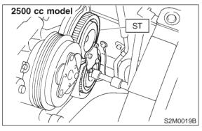
5) Install camshaft position sensor. <Ref. to 2-7 [W10A0].>
