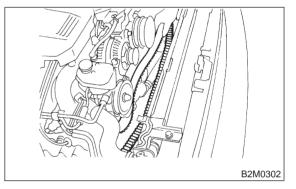
12) Remove automatic belt tension adjuster.
