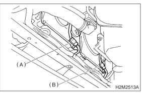
6) Loosen bolts which hold lower side of radiator main fan and sub fan shrouds.
