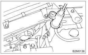
2) Apply a pressure of 157 kPa (1.6 kg/cm<sup>2</sup>, 23 psi) to radiator to check if:
