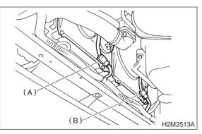
9) Connect radiator outlet hose and water by-pass hose B (AT vehicles).
