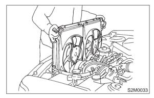
3) Install radiator brackets and tighten bolts.
