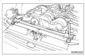
13) While slightly lifting radiator, slide it to left.14) Lift radiator up and away from vehicle.
