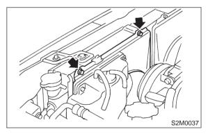
9) Remove radiator main fan motor assembly.
