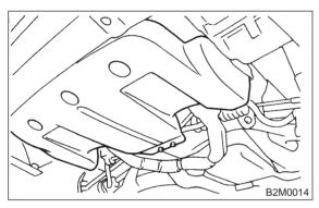
4) Loosen bolts which install the lower side of radiator main fan shroud.
