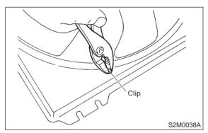
2) Cut band which holds motor harness on shroud.
