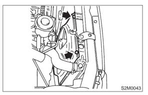
9) Remove radiator sub fan motor assembly.
