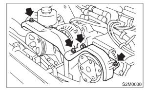
8) Remove bolts which hold sub fan shroud to radiator.
