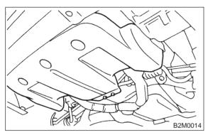
4) Loosen bolts which install the lower side of radiator sub fan shroud.
