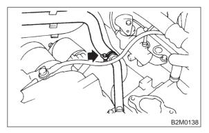
6) Disconnect radiator inlet hose from water pipe.
