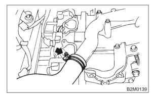
7) Remove bolts which install water pipe on cylinder block.
