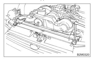
8) Support engine with a lifting device and wire ropes.
