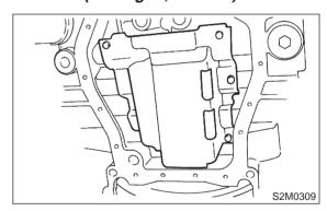
2) Install oil strainer onto baffle plate.
