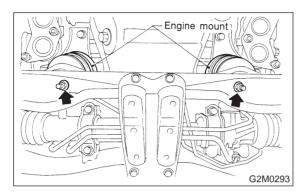
15) Remove bolts which install oil pan on cylinder block while raising up engine.
