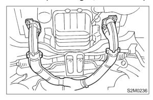
(3) Tighten nuts which install front catalytic converter to center exhaust pipe.
