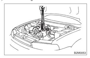
12) Connect connector to front oxygen sensor.
