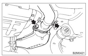
(2) Remove front exhaust pipe from engine.
