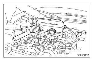
4) Disconnect front oxygen sensor connector.
