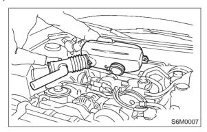
17) Fill engine oil through filler pipe up to upper point of level gauge. <Ref. to 1-5 [G4A0].>
