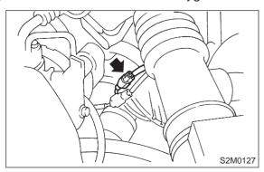
13) Connect connector to rear oxygen sensor. (California spec. vehicles)
