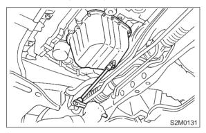
16) Insert oil pan cutter blade between cylinder block-to-oil pan clearance.
