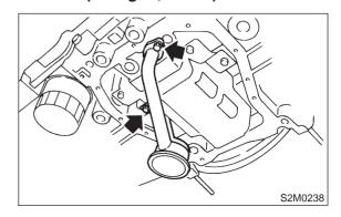
3) Apply fluid packing to mating surfaces and install oil pan.
