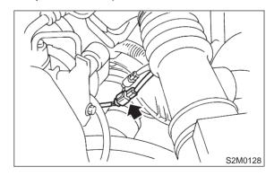
7) Connect front oxygen sensor connector.
