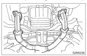
3) Install center exhaust pipe to front exhaust pipe.
