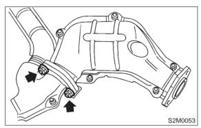
2) Tighten bolts which hold front exhaust pipe onto cylinder heads.
