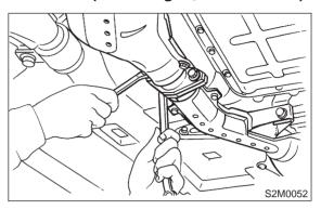
4) Connect rear oxygen sensor connector. (Except California spec. vehicles)
