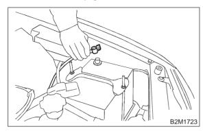
2) Disconnect front oxygen sensor connector.
