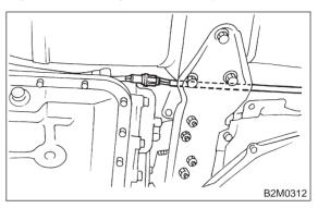
6) Separate center exhaust pipe from front exhaust pipe.
