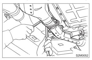
4) Install center exhaust pipe to rear exhaust pipe.
