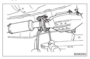
2) Separate rear exhaust pipe from muffler.
