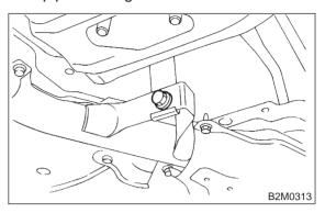
3) Install center exhaust pipe to front catalytic converter.
