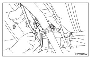
3) Install rear exhaust pipe to center exhaust pipe.
