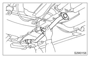
2) Install rear exhaust pipe to muffler.
