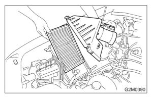
6) Remove mass air flow sensor from air cleaner upper cover.
