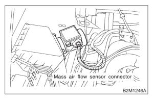
5) Remove two clips, then remove air cleaner upper cover.
