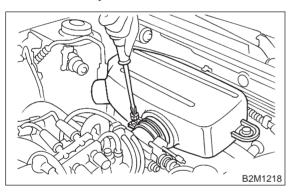
5) Disconnect air hoses, and remove air intake chamber.
