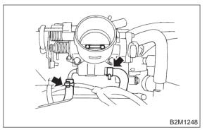
10) Remove bolts which install throttle body to intake manifold.
