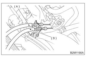
8) Disconnect connector from throttle position sensor.
