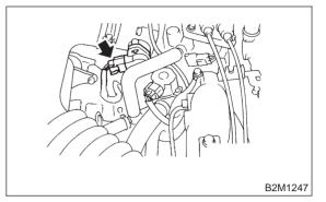
9) Disconnect engine coolant hoses from throttle body.
