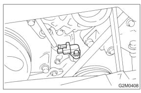
2) Remove crankshaft position sensor, and disconnect connector from it.
