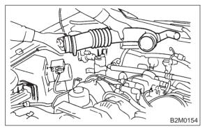
2) Disconnect connector from engine coolant temperature sensor.
