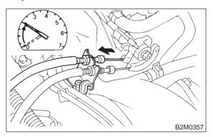
3) Disconnect air by-pass hose from air intake duct.
