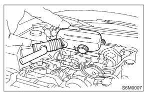
5) Disconnect connector from idle air control solenoid valve.
