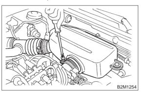
4) Disconnect blow-by hose and air hose, and remove air intake chamber and air intake duct as a unit.
