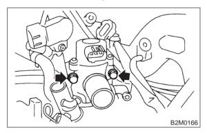
10) Disconnect engine coolant hoses from idle air control solenoid valve, and take them off.
