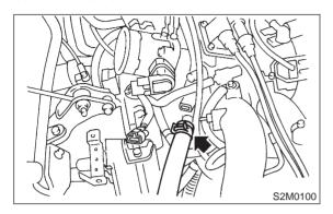
9) Remove bolts which install idle air control solenoid valve to throttle body.
