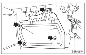
5) Remove vinyl cover and nuts which attach ECM to bracket.
