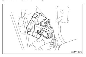
9) Disconnect connector from main relay.
