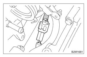
4) Remove knock sensor from cylinder block.
