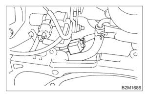
5) Remove knock sensor from cylinder block.
