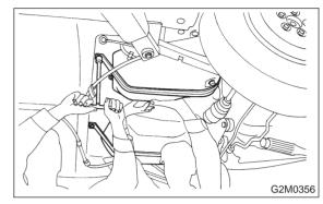
2) Disconnect evaporation hose from fuel cut valve.
