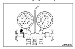
5) After 5 minutes, re-check the low-pressure gauge reading.
