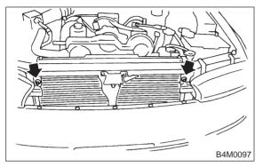
8) The condenser should be installed in the reverse order in which it was removed. When installing the condenser, pay attention to the following:
