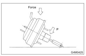
4) Do not change the push rod length. If it has been changed, reset the projected length "L" to the standard length.
