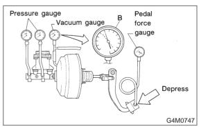
2) Stop engine and watch vacuum gauge. If the vacuum drop range is less than 3.3 kPa (25 mmHg, 0.98 inHg) within 15 seconds after stopping engine, brake booster is functioning properly. If defective, refer to "AIR TIGHTNESS CHECK". <Ref. to 4-4 [W6D2].>
