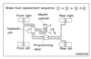
3) Slowly depress the brake pedal and keep it depressed. Then, open the air bleeder to discharge air together with the fluid.
