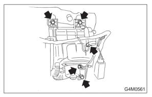
5) Remove screws which secure intake door motor to intake unit.
