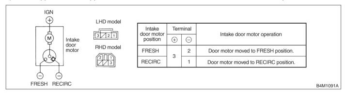
2) Connect harness to intake door motor.
