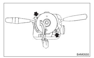
2) Fit upper column cover to lower column cover, and tighten combination switch and column cover.
