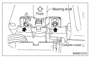
9) Pull out steering shaft assembly from hole on toe board.
