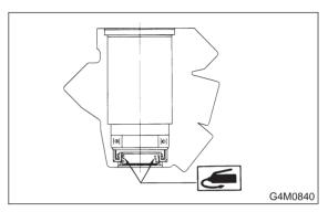
7) Apply a coat of specified steering grease to ST surface, and install ST onto end of input shaft. Insert pinion and valve until "A" of oil seal contacts "B" of valve housing. The ST is used to prevent scratching Y-packing.
