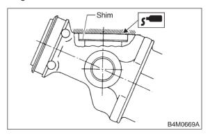
3) Use the same number of shims as that used when steering body was removed.
