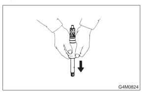
2) Using ST and press, remove dust seal, back-up washer, Y-packing and ball bearing from valve housing.
