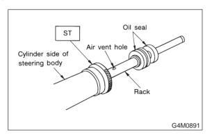
6) Slowly press inner side oil seal until distance between ST and end of rack is 65 mm (2.56 in). ST 34099FA010 GUIDE (Oil seal)
