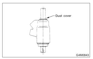
10) Adjust sealing lip-to-housing end clearance to 0 to 0.5 mm (0 to 0.020 in). If sealing lip is too close to housing end, steering wheel will not return smoothly; if it is too far from housing end, dust or dirt will enter the clearance.
