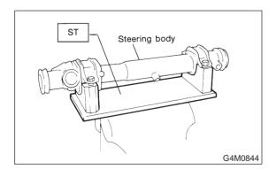
2) Using ST-B and ST-C, attach oil seal to ST-A. Insert ST-A into rack from gear side. Remove oil seal from ST-A when it approaches piston and remove STs from rack.
