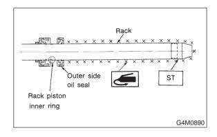
5) Apply a coat of grease to grooves in rack, sliding surface of sleeve and sealing surface of piston. Install ST on the end of steering body cylinder. Then insert rack into steering body from cylinder side.
