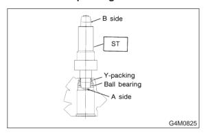
3) Apply a coat of grease to inner wall of valve housing, Y-packing and outer perimeter of dust seal.
