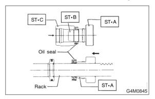
3) Install back-up ring from gear side of rack.
