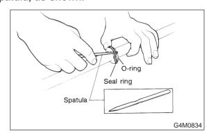
4) Apply a coat of grease to inner surface of ST and insert rack piston into it. Leave ST at least 10 minutes until seal ring settles down in place. ST 927600000 FORMER
