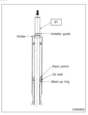
10) Using ST, clinch steering body cylinder at a point less than 3 mm (0.12 in) from holder.
