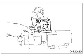
9) Attach ST to rack cylinder. Using a press, install back-up ring and oil seal.
