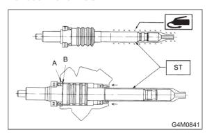
8) While supporting pinion and valve, push end of pinion until bearing contacts brazed end of valve housing.
