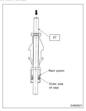
3) Insert ST from valve side and press back-up ring and oil seal out.
