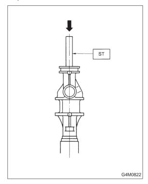
4) Using ST1 and ST2, repair cylinder's clinched sections.
