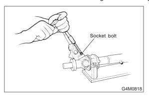
3) Remove valve housing, pinion and valve as a unit.
