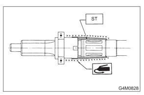
6) Apply a coat of grease to spacer and sealing lips of oil seal, and install spacer and oil seal.
