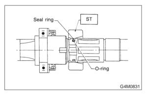
9) While aligning valve sleeve pin with groove on pinion, secure with snap ring.
