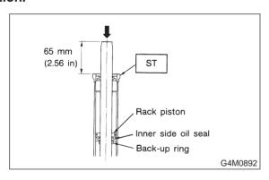
7) Pass ST2 and pipe through rack and press outer side oil seal until ST1 is in contact with ST2.
