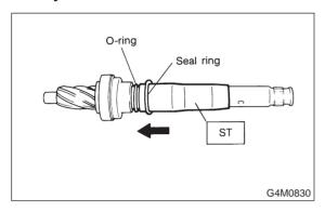
8) Apply a coat of grease to inner wall of ST, and secure seal ring assembled in former step as shown. Leave seal ring unattended for approximately 10 minutes until it settles down.
