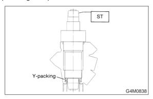
5) Attach ST2 to ST1, and press ball bearing into place using a press.
