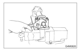
2) Install ST on valve side of rack and press outer side oil seal out.
