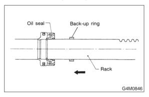
4) Install ST on rack and equally apply a thin coat of grease to rack and ST, then install oil seal. ST 926250000 GUIDE
