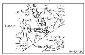
5) Remove flare nuts from control valve of gear-box assembly, and then disconnect pipe C·D.
