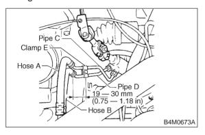
6) Temporarily install clamp E on pipes C and D.
