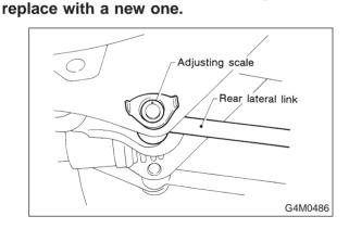
2) Turn adjusting bolt head until toe-in is at the specification.
