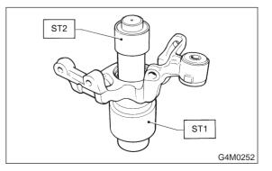
6) Remove tone wheel bolts and remove tone wheel from hub (only vehicle equipped with ABS).7) Using ST, press hub bolts out.
