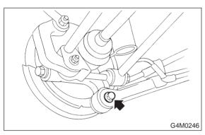
10) Remove bolts which secure lateral link assembly to rear housing.
