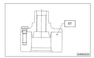
2) Remove foreign particles (dust, rust, etc.) from mating surfaces of hub and tone wheel, and install tone wheel to hub (only vehicle equipped with ABS).
