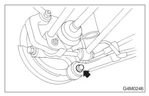
11) Remove bolts which secure lateral link assembly to rear housing.
