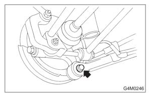
5) Connect parking brake cable to parking brake.
