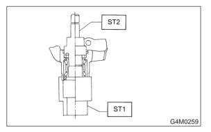
8) Using ST1 and ST2, press sub seal into place.
