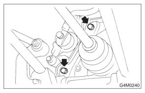
8) Install rear speed sensor to back plate (only vehicle equipped with ABS).
