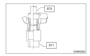
9) Apply sufficient grease to oil seal lip.
