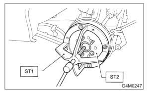
12) Remove rear ABS sensor from back plate (only vehicle equipped with ABS).
