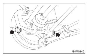
11) Disengage BJ from housing splines, and remove rear drive shaft assembly. If it is hard to remove, use STs.
