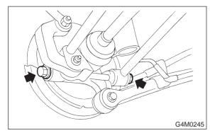
4) Connect rear housing assembly to trailing link assembly.
