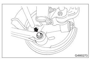
11) Remove bolts which secure lateral link assembly to rear spindle.
