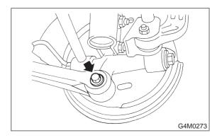
12) Remove bolts which secure lateral link assembly to rear spindle.
