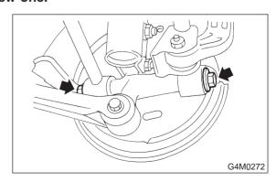
12) Remove bolts which secure strut assembly to rear spindle.
