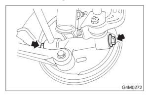
3) Connect rear spindle assembly to trailing link assembly.
