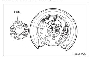
2) Remove back plate from rear spindle.
