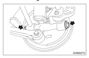
3) Connect rear spindle assembly to trailing link assembly.
