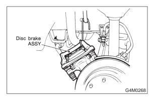
8) Remove disc rotor from hub.
