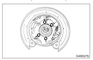
3) Using ST, press hub bolts out.
