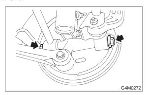
13) Remove bolts which secure strut assembly to rear spindle.
