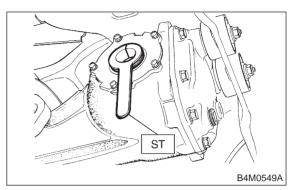
4) Insert DOJ spline end into bore of side oil seal, and remove ST.
