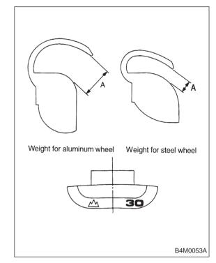
Service limit: A Weight for steel wheel; 1.6 — 2.0 mm (0.063 — 0.079 in) Weight for aluminum wheel; 4.6 — 5.4 mm (0.181 — 0.213 in)
