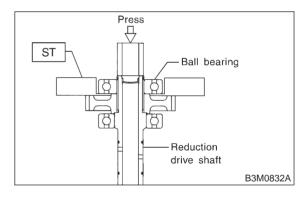
4) Using a press, remove the reduction drive gear.
