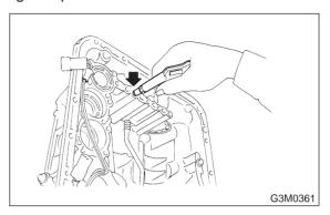
25) After removing the snap ring (inner) using ST1 and ST2, take out the servo piston by applying compressed air from the release pressure side.
