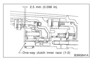
14) Assemble the overrunning clutch hub.
