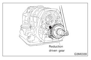
4) Install the reduction drive gear assembly.
