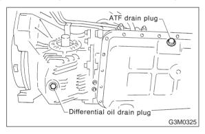
3) Remove the drain plug, and drain automatic transmission fluid (ATF). Tighten the plug temporarily after draining.
