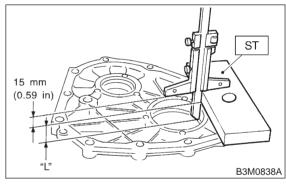
(2) Measure distance  $\ell$  from end of transmission case to end of bearing.
