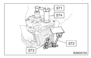
(8) Apply red lead evenly to the surfaces of three or four teeth of the crown gear. Rotate the drive pinion in the forward and reverse directions several times. Then remove the oil pump housing, and check the tooth contact pattern. If tooth contact is improper, readjust the backlash or shim thickness.
