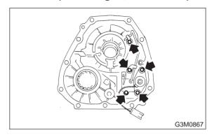
3) Install the transfer clutch assembly to the case.
