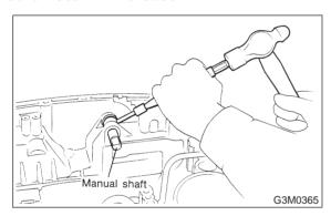
30) Remove the inhibitor switch.
