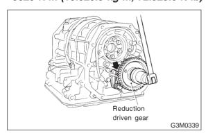
5) Install the reduction drive gear assembly.
