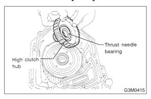
22) Install the high clutch assembly.
