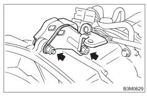
9) Tighten the drain plugs.
