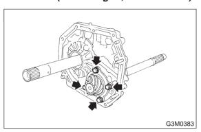
(3) Install the oil pump housing assembly to the torque converter clutch case, and secure evenly by tightening four bolts.
