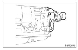
7) Install the vehicle speed sensor 1.
