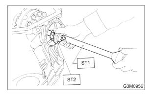
4) Remove the differential case assembly.
