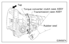
2) Separation of transmission case and transmission cover
