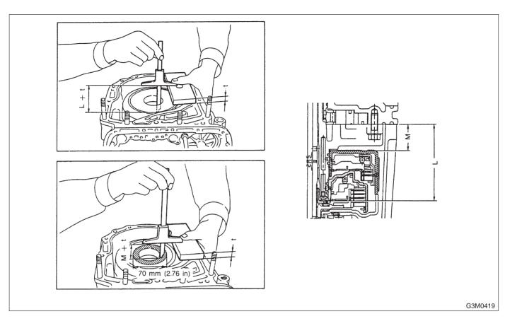
(2) Measure the distance from the oil pump housing mating surface to the top surface of the
