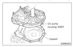
(4) Secure the housing with two nuts.
