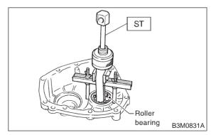
4) Take out the roller bearing outer race with ST.
