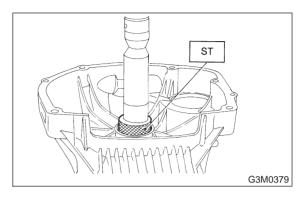
6) Install the differential assembly to the case, paying special attention not to damage the speed-ometer gears (drive and driven) and the inside of the case (particularly, the differential side retainer contact surface).
