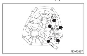
3) Take out the roller bearing inner race with ST. ST 398527700 PULLER
