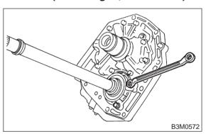
16) Apply vaseline to the groove on the oil pump cover, and install two (R) seal rings and two (H) seal rings.
