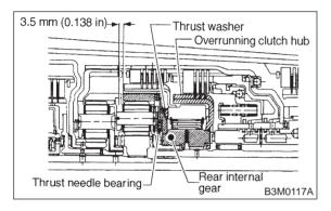
17) Install the rear planetary carrier.
