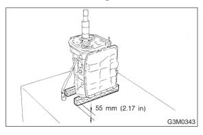
6) Remove the oil pan and gasket.
