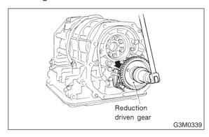
(2) Using the ST, extract the reduction driven gear.
