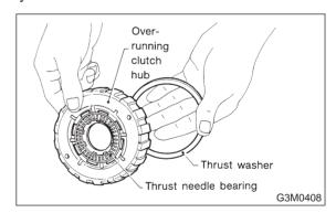
15) Install the one-way clutch outer race.
