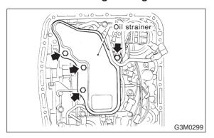
10) Remove the control valve body and the two brackets.
