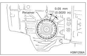
(7) Turn the drive pinion several rotations with ST1 and check to see if the backlash is within the standard value with ST2, ST3 and ST4.
