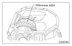
7) Install the circlip to the axle shaft, insert the shaft into the differential assembly, and tap it into position with a plastic hammer.
