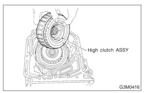
23) Install the reverse clutch assembly.
