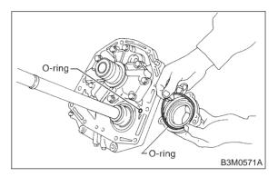
15) Install the oil seal retainer taking care not to damage the oil seal lips. Then secure with three bolts.
