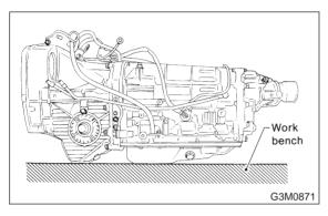
2) Remove the drain plug, and drain differential oil. Tighten the plug temporarily after draining.
