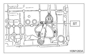
(2) With hole aligned, tighten three bolts to secure the inhibitor switch.
