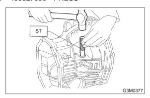
3) Install vehicle speed sensor 2.
