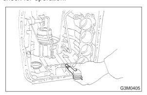
(3) Check the clearance. (Selection of retaining plate)
