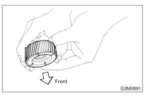
19) Install the front planetary carrier.
