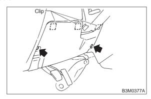
3) Remove transmission control module.
