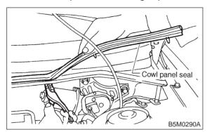
4) Lift cowl panel and detach it from clips attached to body panel.
