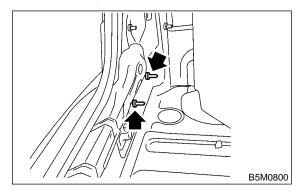
5) Remove eight clips and then disconnect upper beam (A) from bumper face (B).
