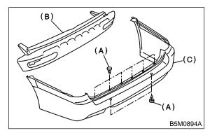
7) Disconnect resin beam from bumper beam.
