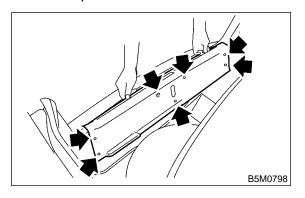
3) Remove hook (A) and then turn over the trunk side trim of the rear portion.
