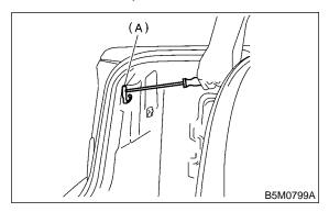
4) Remove two nuts of both sides and then detach bumper assembly.
