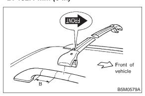
3) Rotate the lower clamp up to the bottom of the roof rail and loose assemble the TORX bolt T30, through the top of the end support and into the threaded insert in the lower clamp on each end of the crossbar.
