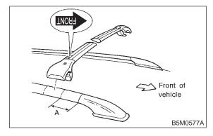
3) Rotate the lower clamp up to the bottom of the roof rail and loose assemble the TORX bolt T30, through the top of the end support and into the threaded insert in the lower clamp on each end of the crossbar.
