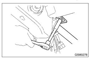
13) Set temperature control switch (A) to "FULL HOT" and then disconnect temperature control cable from bottom of heater unit.
