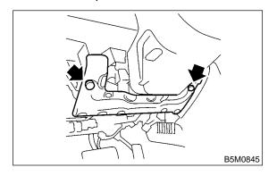
5) Remove stopper (A) and then remove glove box.
