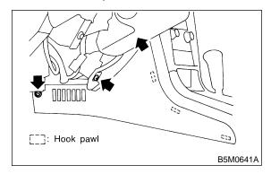
7) Remove tray (A) and console cover (B) while disconnecting connector.
