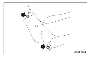
10) Remove front seat from vehicle, then install headrest.
