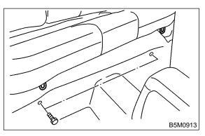
2) Slightly raise front of cushion while pushing down on cushion in the direction of "A". With cushion held in that position, move it forward until it is unhooked.
