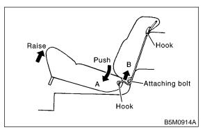
3) Remove bolts securing lower portion of backrest and then open the center trunk through lid.
