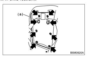
3) Remove screws and then detach cushion board (a).
