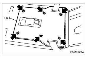
4) Remove screws and then detach retractor assembly (a).
