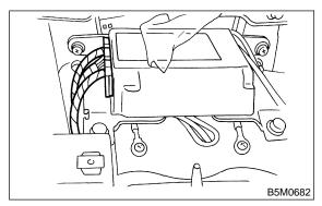
7) Disconnect body harness connector (B31) from airbag connector (AB1) located in front pillar lower (driver side). <Ref. to 5-5 [M2F3].>
