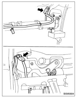
9) Detach clips from steering support beam and remove main harness.
