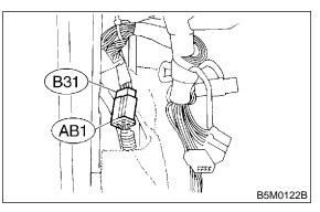
8) Disconnect front sub sensor connector (blue) from airbag main harness. <Ref. to 5-5 [M2F2].>
