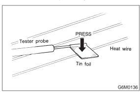
4) When tester indicates 12 volts when its probe reaches point "A", a broken circuit occurs between point "A" and the negative terminal. Slowly move tester probe toward the negative terminal while contacting it on heat wire to locate point where tester indication changes abruptly (0 volts). This is the point where a broken circuit occurs.
