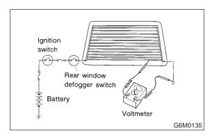
• When measuring voltage, wind a piece of tin foil around the tip of the tester probe and press the foil against the wire with your finger.
