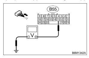
: Is the voltage less than 1  $V \leftarrow \rightarrow$  more (CHECK) than 4 V?
