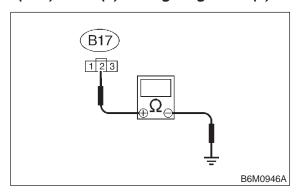
$\widehat{\text{CHECK}}$ : Is the resistance less than 10  $\Omega$ ?
