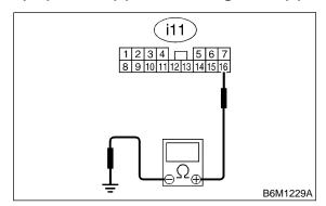
$\widehat{CHECK}$ : Is the resistance less than 10  $\Omega$ ?
