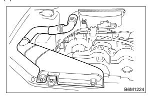
(4) Remove resonator chamber.
