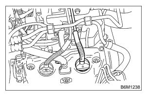
4) Remove spark plug with the spark plug socket.
