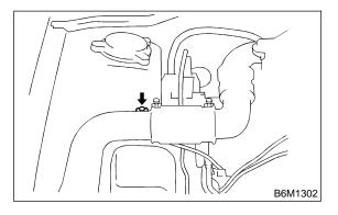
(3) Remove air intake duct as a unit.
