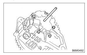
When installing rear cover, heat portion (A) to 50°C (122°F) with heater drier.
