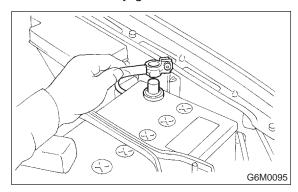
2) Disconnect washer motor connector.
