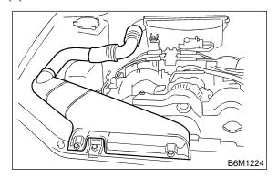
(4) Remove resonator chamber.
