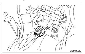
4) Remove ignition coil and ignitor assembly.
