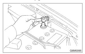
2) Disconnect spark plug cords from ignition coil and ignitor assembly.
