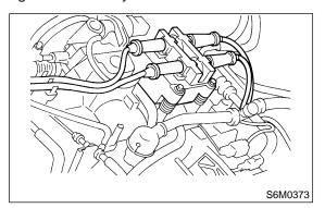
3) Disconnect connector from ignition coil and ignitor assembly.
