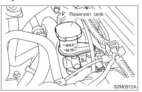
2) Make sure that brake fluid does not leak from master cylinder, operating cylinder and piping.
