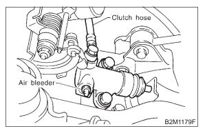
3) Slowly depress the clutch pedal and keep it depressed. Then open the air bleeder to discharge air together with the fluid.
