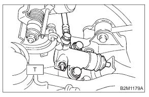
6) After depressing the clutch pedal, make sure that there are no leaks evident in the entire system.7) After bleeding air from system, ensure that clutch operates properly.
