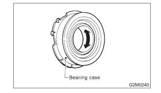
3) Check wear and damage of bearing case surface contacting with lever.
