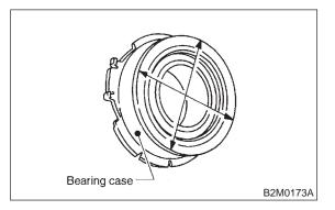
2) Check the bearing for smooth rotation by applying pressure in the thrust direction.
